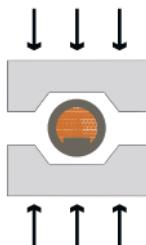
Fix the lug in the corresponding tool matrix and make pressing (crimping), as far as it will go.
