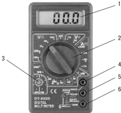
1 – 3 ½ digits LCD, height of characters is 12.7 mm. Display shows measurement results in digital form.
